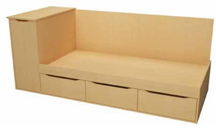
The premium student beds come with an 18mm MFC carcass with 2mm PVC edging. The beds include a cupboard headboard, wall protector and 3 under bed drawers on 40kg ball bearing runners with scalloped handles.
